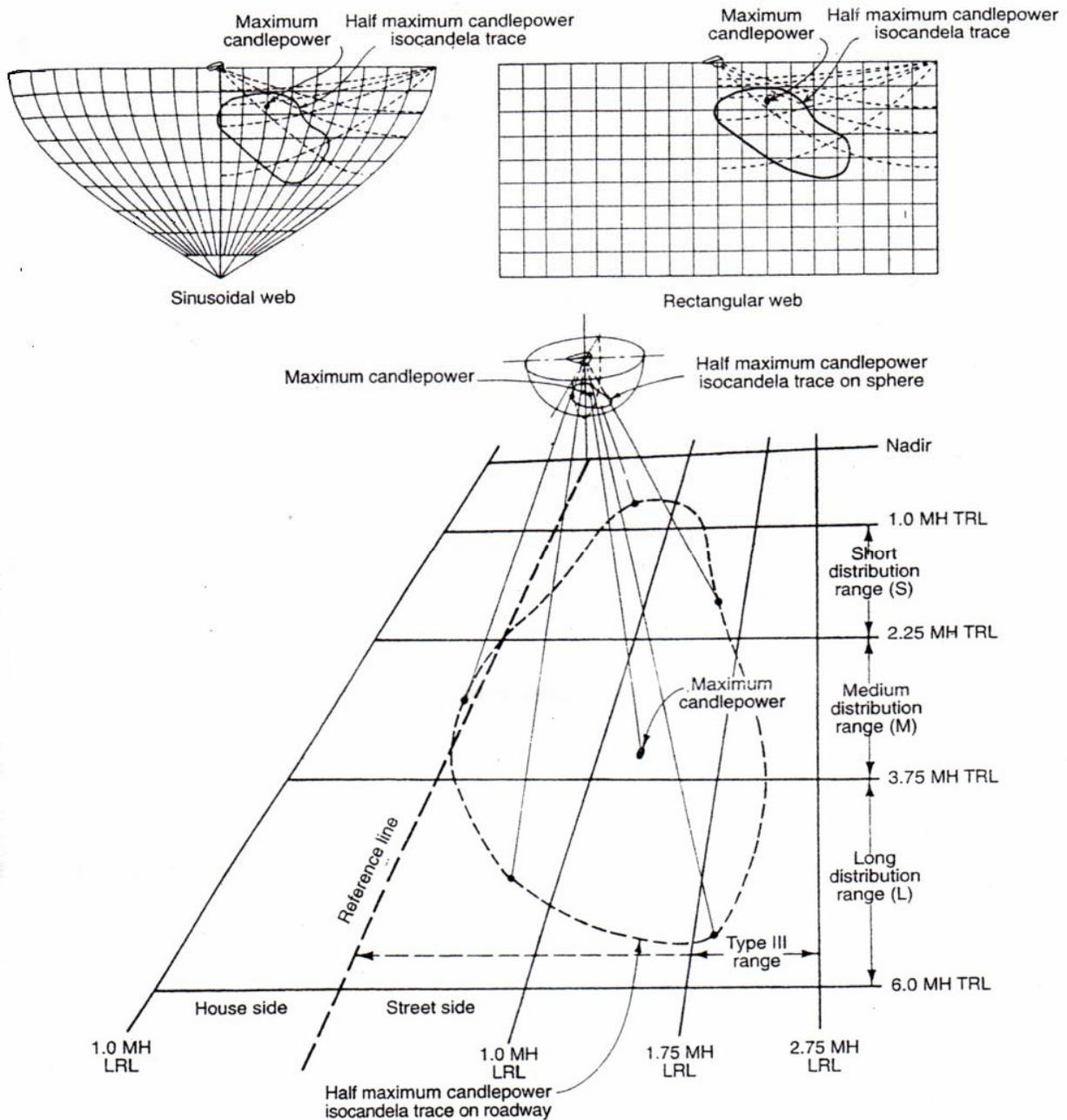
**Figure 22-7.** Diagram showing projection of maximum candlepower and half-maximum candlepower isocandela trace from a luminaire having a Type III-Medium distribution, on the imaginary sphere and the roadway. Sinusoidal web and rectangular web representation of sphere are also shown with maximum candlepower and half-maximum candlepower isocandela trace.
