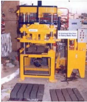
**Figure 6** *Bricks and Blocks manufacturing machine*
