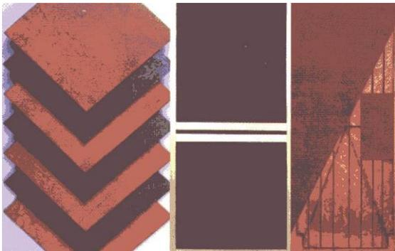
**Figure 15** *Red Mud Based Composite Products tiles, boards and shutter from L to R)*
