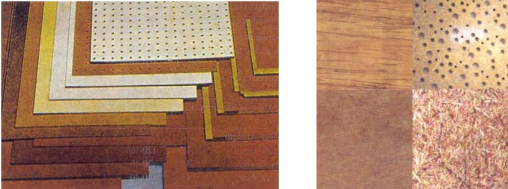
**Figure 16** *Bagasse Board (left) and Agro-waste recycled boards ( right)*
