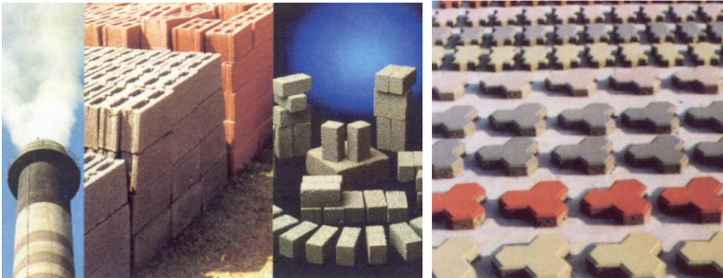
***Figure 5*** Fly Ash Based Bricks and Blocks
