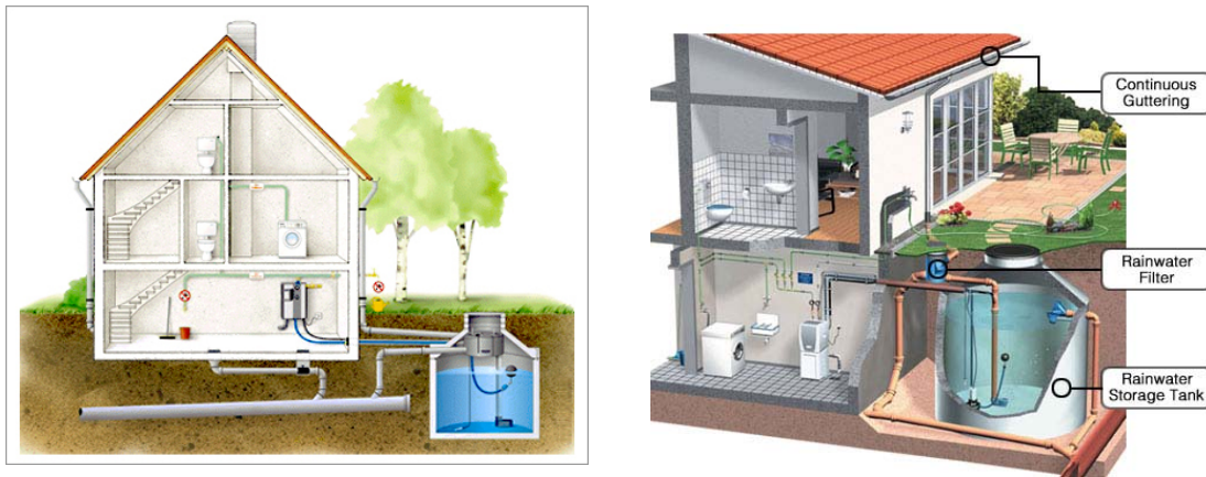
Figure 1. Roof Top Rain Water Harvesting for direct storage and use (Non Potable use)
