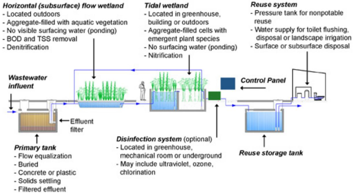
Figure 3. Working of Hybrid wetland system, Source: [www.livingmachines.com](http://www.livingmachines.com)
